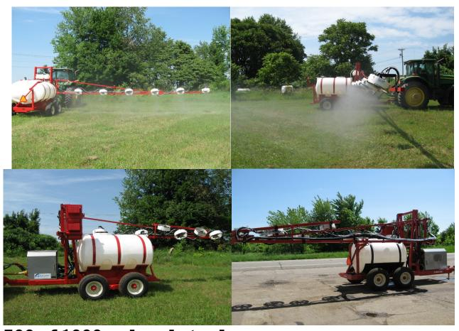
500 of 1000 gal. poly tank **Heavy duty frame** Heavy duty one side folding boom With six Proptec heads Walking beam suspension **Self Contained Power Pack** Stainless Shroud
