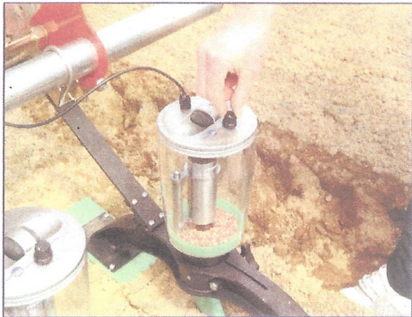
12 volt DC supply Set the seeding rate with the turn of a dial
