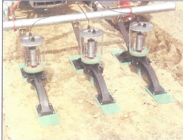
Abrasive resistant plastic skids level the seed bed and cover the placed seed
