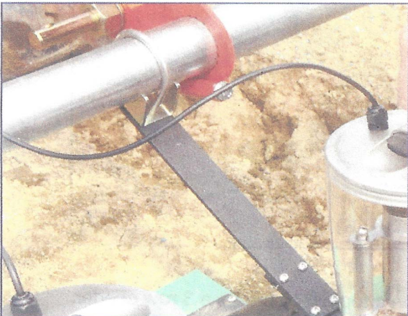
Spring steel arm connection to the toolbar allows the Rocket to contour follow
