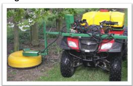
The Spraydome is made of durable plastic. The most common size is a 600mm (24"). Other sizes include 400 (18"), 1000 (39") and the 1200 (48").
